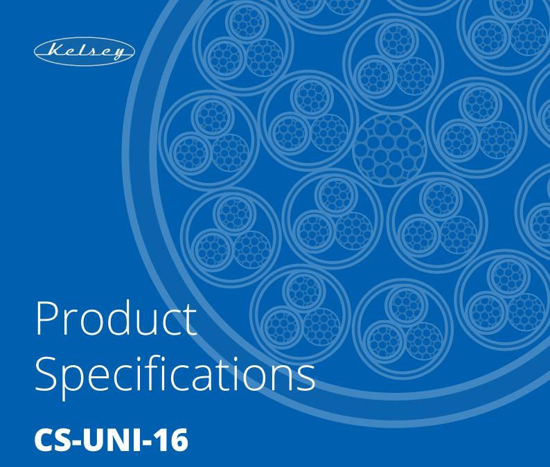
**Kelsey's Universal Contractor Series** has been designed to offer the excellent performance of the Universal series with an LSZH jacket for compliance with installation legislation in public areas. Adopting the particular characteristics of the Universal series, each foil-screened twisted pair is individually jacketed and shielded to create a durable multipair cable that can be implemented for both analogue and digital as well as DMX applications.
